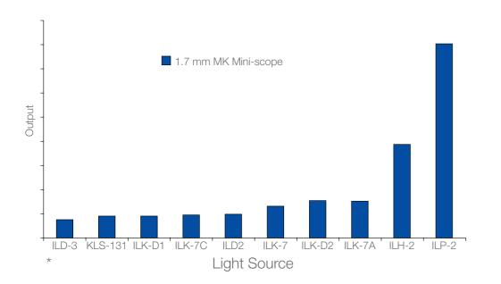
\* Brightness comparison measurements taken at the tip of the scopes
